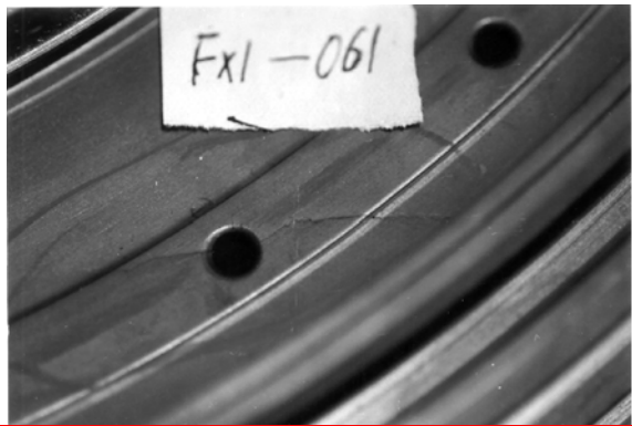
图3 修理中发现的孔边裂纹 Fig. 3 Crack found in repairation
